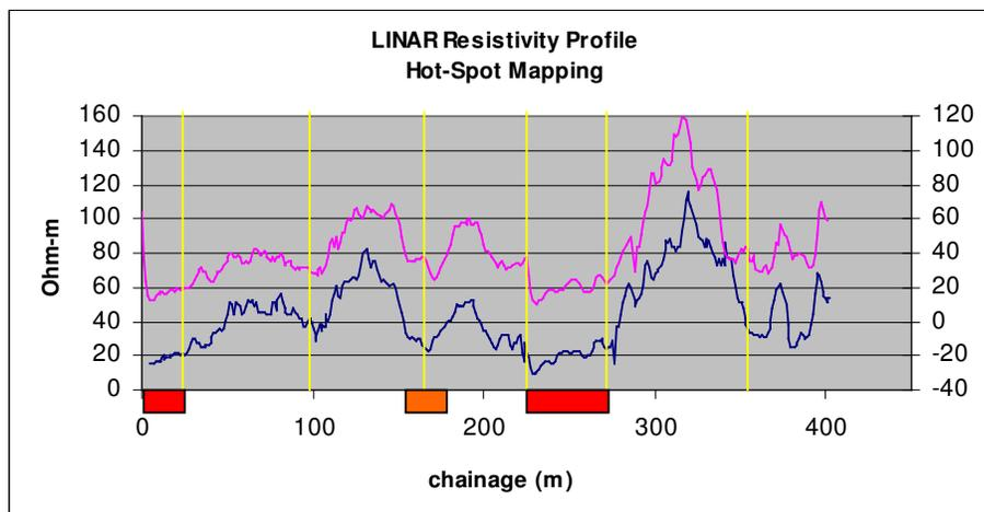
Figure 1 : LINAR resistivity profile indicating "hot-spot" corrosion for LPR extrapolation.
