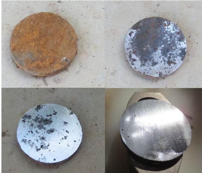
**Fig 1. Progressive polishing of coupon samples (following 11 mth burial) from (a) as exhumed, (b) oxide removal, (c) moderate pitting, (d) remanent deep pits close to total removal. Pit depths calculated from weight loss through polishing.**
