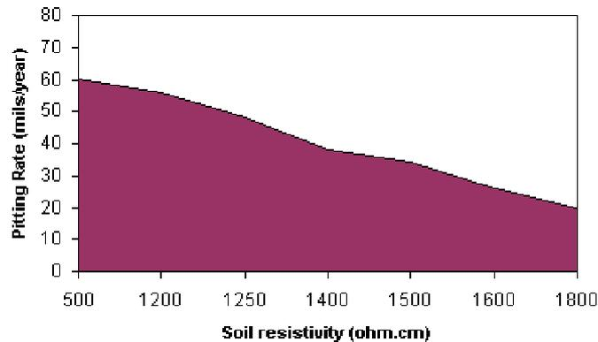
Soils of low resistivity are also likely to cause more rapid pitting attacks on ductile iron at rates that increase as the resistivity decreases. The shaded area in this Figure gives a typical range for the average maximum pitting rates for ductile iron pipe as a function of soil resistivity. It is compiled from data found by various surveys and studies done in the U.S., Canada and Europe.
