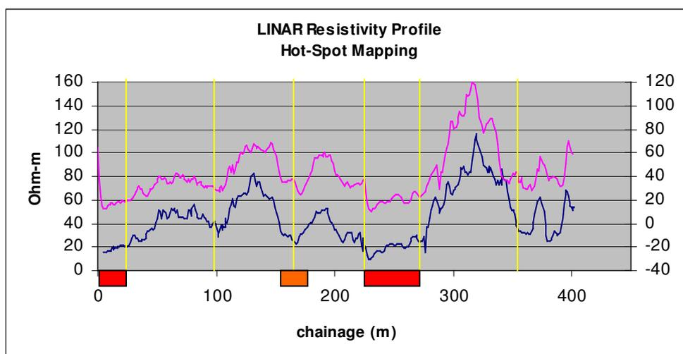
**LINAR resistivity profiles indicating potential corrosion “hot-spots” and lateral variations in soil condition. Two traces from separate surveys indicating consistent response in urban setting.**
